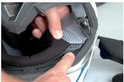
➡ B. Insert the maximum of hard rear part between the shell and polystyrene. Attention : not to deteriorate the polystyrene.
