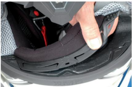
➡ A. Slide the front in its support. The clips must be correctly locked. Clip the 2 snaps holding the rear of the cap.
