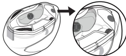
Place the external button on the left side of your helmet using the 3M adhesive already on it.
