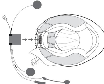
Connect the two speakers to the plug B and C. Place both speakers in the deep ear pocket of your helmet. You can fix the speakers using the velcro pad supplied in the box.
