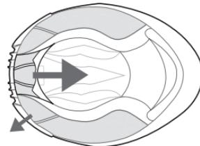
Insert the Bluetooth box well deep in the place, only the cables must be outside.
