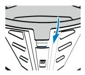
3- To completely close the visor, lower it until reaching the locking position.
