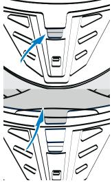
2- Lower the visor once again in placing it against the button without applying any force.
