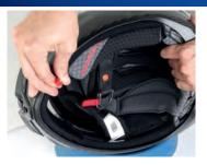
4 - Unfasten the snaps at the back of the peak and then withdraw the front plastic part from its slot. Remove the peak.
