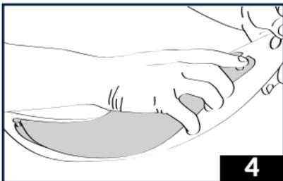
4 - Extend and flex the visor and fit the second side of the PINLOCK® lens into the second pin. Release the visor so that it reacquires its curved shape.
