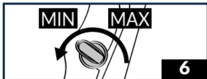
6 - Turn the 2 levers outwards to increase the tension of the lens (rotate towards «MAX»).
