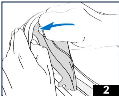
2 - Slide the central plastic backing of the breath guard between the shell and the EPS.
